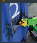
The operation of the machine is very convenient. The travelling length can be programmed quickly and easily for different container lengths using a multi-function joystick. The traction drive is equipped as standard with two electric wheel motors, which are also steplessly controlled via the joystick and an electronic
